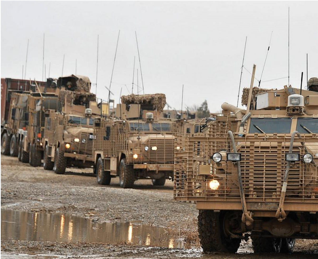
Figure 1: An Army Convoy of Vehicles each with a Number of Omnidirectional Whip Antennas
