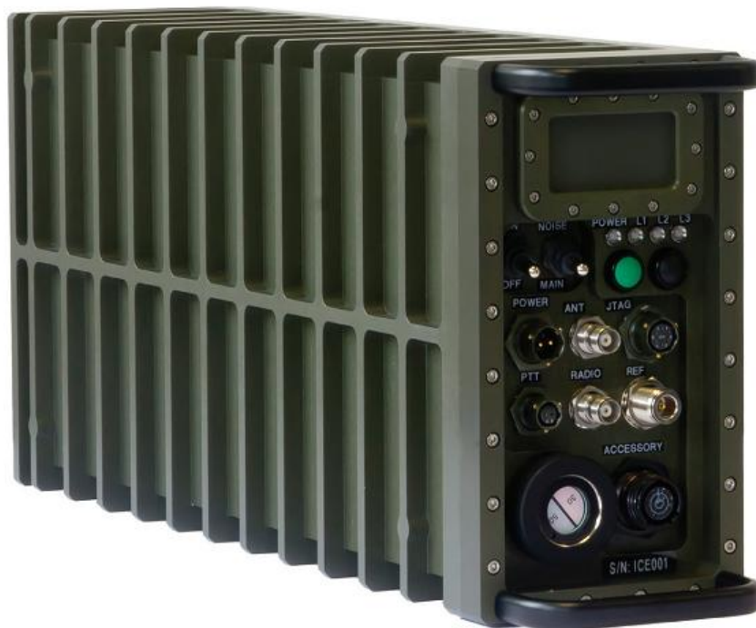
Figure 12: RF Interference Cancellation System to remove Main Large Comms Signal and Sideband Noise
