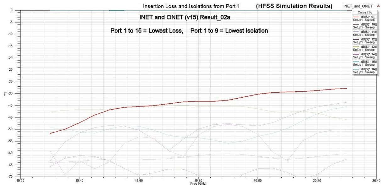
The measured results on the INET connected to the ONET through eight phase matched waveguide channels were plotted over a wider frequency range to show the lower limit for
