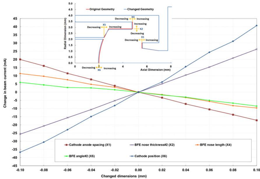
**Figure 5: Electron gun tolerance analysis**
