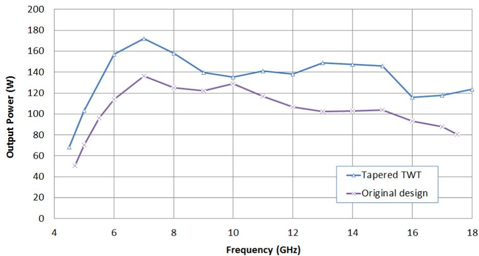
**Figure 4: Broadband performance enhancement via helix pitch profiling**
