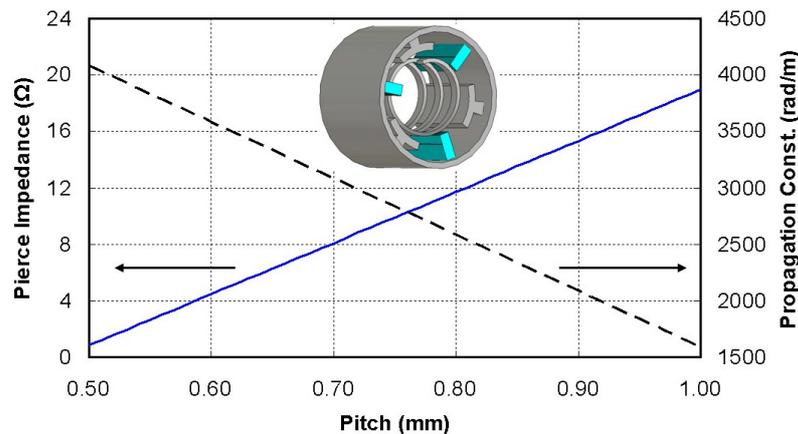
**Figure 3: Variation of Pierce impedance and propagation constant with helix pitch at 18GHz**
