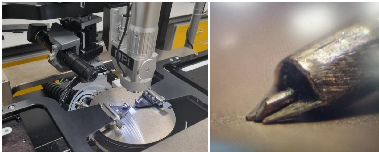
Figure 2 a) Side-view camera installation on the NPL probe station b) magnified image of probe tip landed on gold substrate captured by side-view camera
