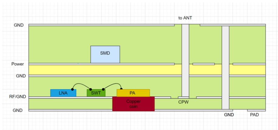
Figure 6 : Stack up for embedded die in PCB
