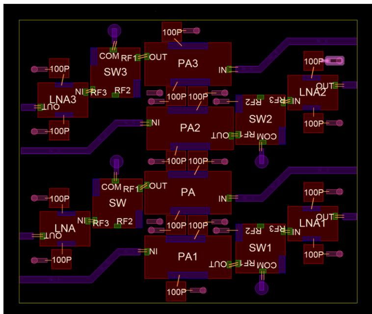
Figure 1 : integration plan for phased array
