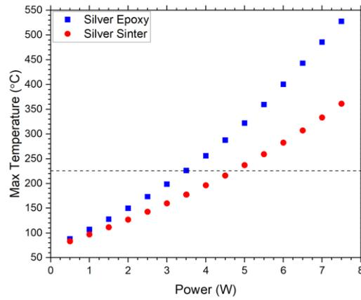
Figure 2: thermal simulation for silver epoxy and silver sintering.
