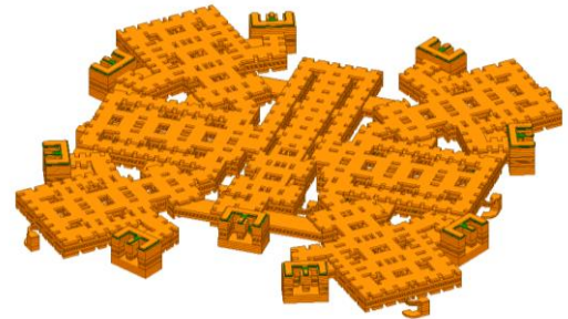
Figure 1. Full 3D layout of proposed eight-way divider
