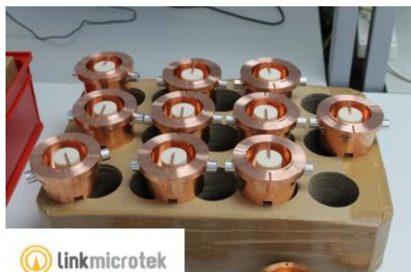
Fig.2: EMILI 2S bottle scanner with integrated weight sensor (left) and dual-mode cavity small scale manufacturing at Link Microtek in Basingstoke (right).
