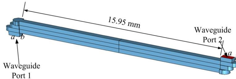
Figure 1: 3D EM model for the WR-3 waveguide with bends. Here the inside of the metal waveguide is shown in blue and the layers are clearly seen.
