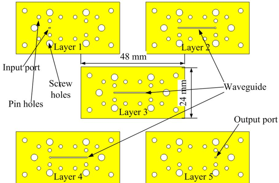
Figure 4: The SU-8 layers for the WR-3 waveguide.
