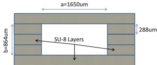
Figure 2: Structure and Dimensions of 150 GHz waveguide
