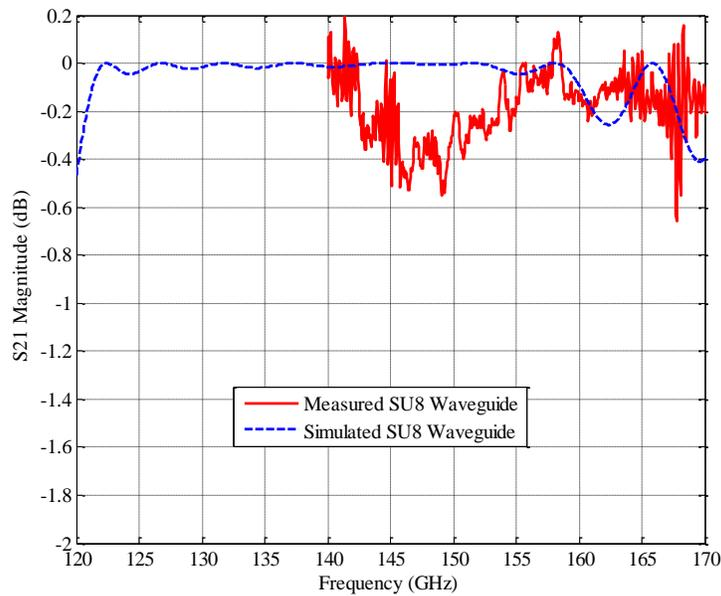
Figure 10:  $S_{21}$  Results of 150 GHz waveguide
