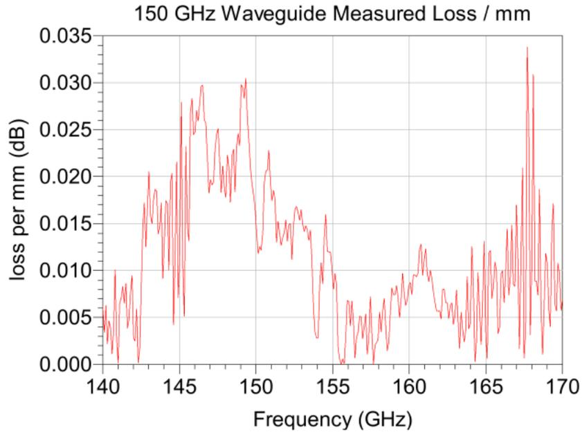
Figure 11: Insertion Loss per mm for 150 GHz waveguide
