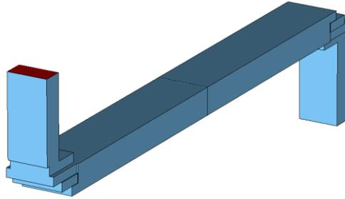
Figure 3: 3D Model of 150 GHz Waveguide and bends
