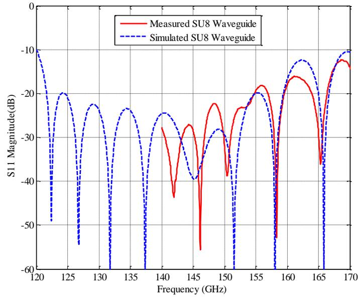
Figure 9:  $S_{11}$  Results of 150 GHz waveguide
