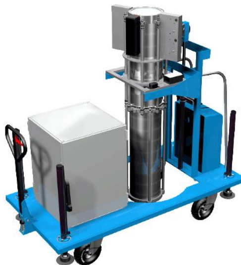
Figure 5 CAD model of gravity sensor being developed at Teledyne e2v for subterranean surveying.
