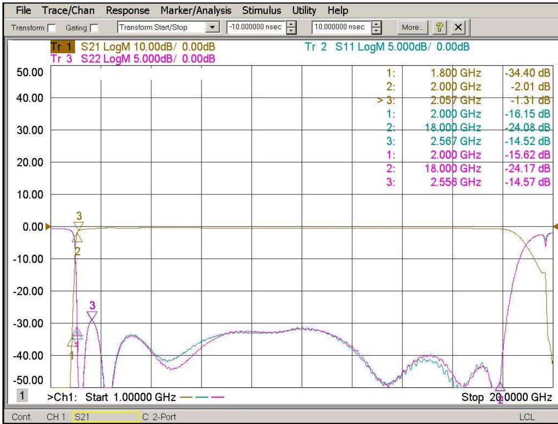
Figure 7 Measured response of the elliptic filter.
