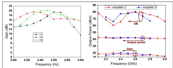
Fig. 4. (a)The measured small signal gain of the designed narrowband amplifiers with frequency. (b) The measured output power, gain, and drain efficiency (DE) of the amplifiers (Amplifier 2 and amplifier 3) with frequency.
