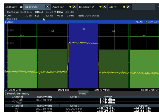
Figure 6 – ACPR performance at Reference input power
