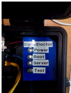
Figure 19: Photo of the RF Front End Status Panel
