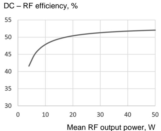
Figure 3 Predicted efficiency versus mean RF output power
