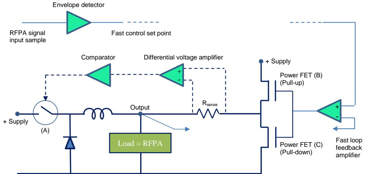
Figure 2 Complete drain bias modulator (simplified)
