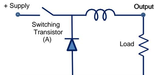
Figure 1 Elementary buck converter
