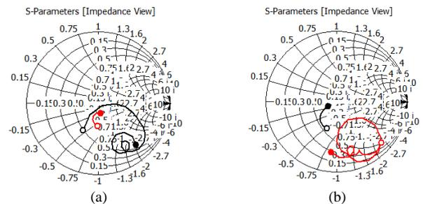
Fig. 3. Impedance match under unloaded and loaded conditions (2.445-2.455 GHz), a) port 2, b) port 4.
