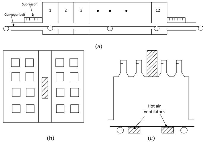
Fig. 1 System configuration, a) running belt and chambers, b) top view of a chamber, c) side view of a chamber.
