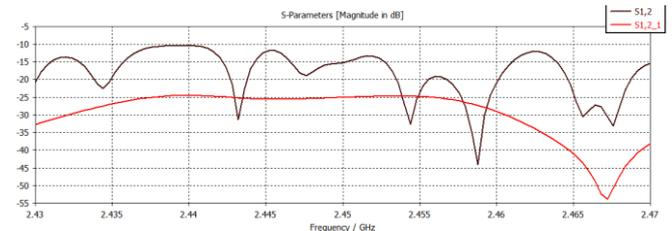
Fig. 4. Magnetron port 1 to port 1 coupling, unloaded (black), loaded (red).
