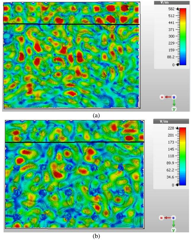
Fig. 2. Electric field distribution at product plane, a) unloaded, b) loaded.
