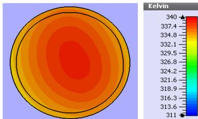
Fig. 5. Temperature distribution inside the fig at  $t = 12$  ms (all magnetrons operating and  $T_0 = 273$  K).
