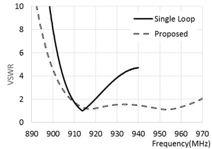
Figure 12. :- VSWR measurements 0.085 l of water – load
