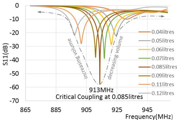
Figure 5:- Reflection coefficient measurements 0.085-0.12 l of water – load.
