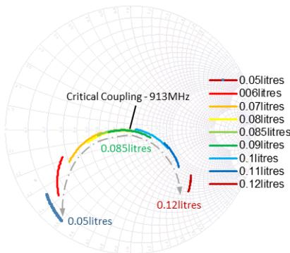
Figure 4:- Impedance variations due to changes in load 0.085-0.12 l of water – load.
