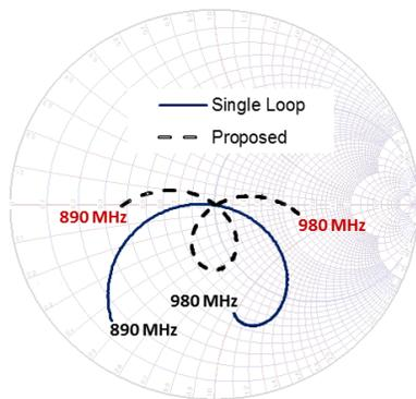
Figure 10:- Coupling with single loop and proposed approach - 0.085 l of water – load.
