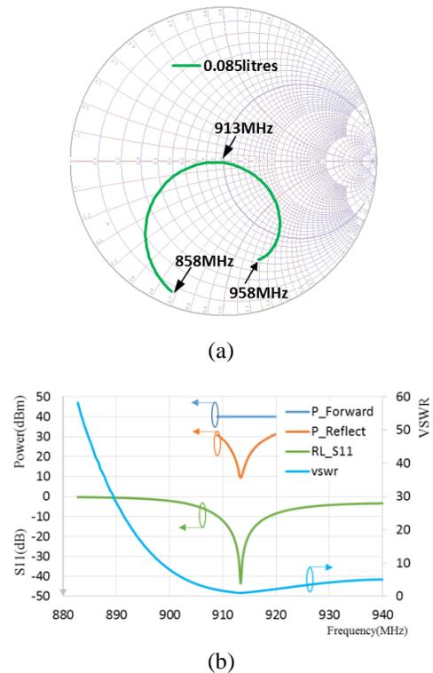
Figure 2: - Critical Coupling at 913 MHz with a single loop coupling structure - 0.085 l of water.
