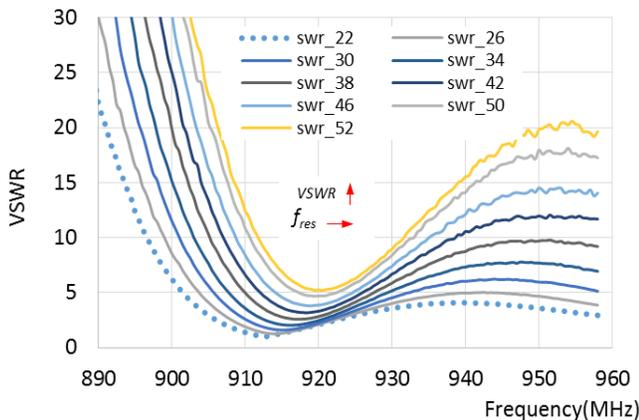
Figure 9:- VSWR measurements 0.085-0.12 l of water – load.
