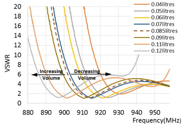
Figure 6:- VSWR measurements 0.085-0.12 l of water – load.
