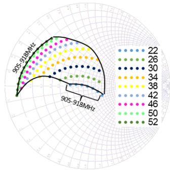
Figure 7:- Impedance variations due to changes in temperature 0.085 l of water – load.
