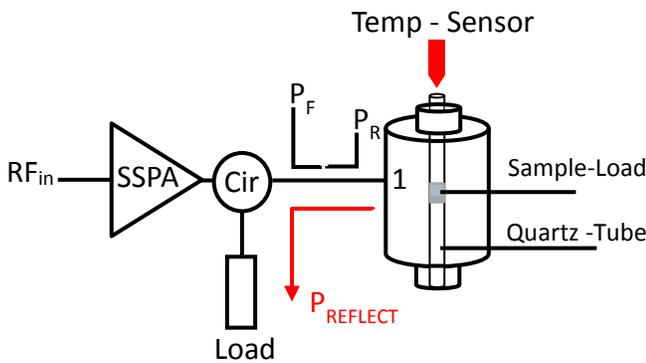
Fig.1. Single Port Measurement Set-up
