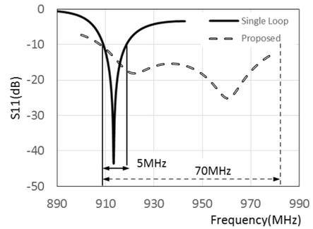
Figure 11:- Reflection coefficient measurements for the two coupling structures for 0.085 l of water – load.
