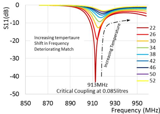
Figure 8:- Reflection coefficient measurements with temperature variations (°C) - 0.085 l of water – load.
