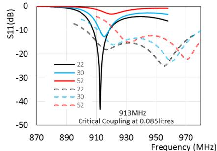
Figure. 15:  $S_{11}$  (single mode vs proposed) with temperature (22°C, 30°C and 52°C) - 0.085litres of water – load
