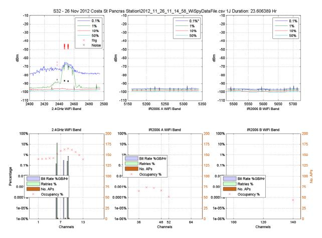
Spectrum analyser data for the three WiFi bands was plotted at the top while the corresponding statistics from WiFi radio header was plotted below. In addition WiFi signal levels were superimposed on the spectrum analyser plots and occupancy (derived from spectrum analyser data) was superimposed over the WiFi metrics.
