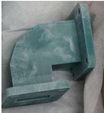
Fig 2 WG16/WR90 Bend printed in wax
