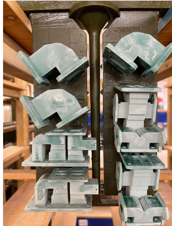
Fig 3 Various 3d printed waxes assembled on the “tree” ready for investment casting
