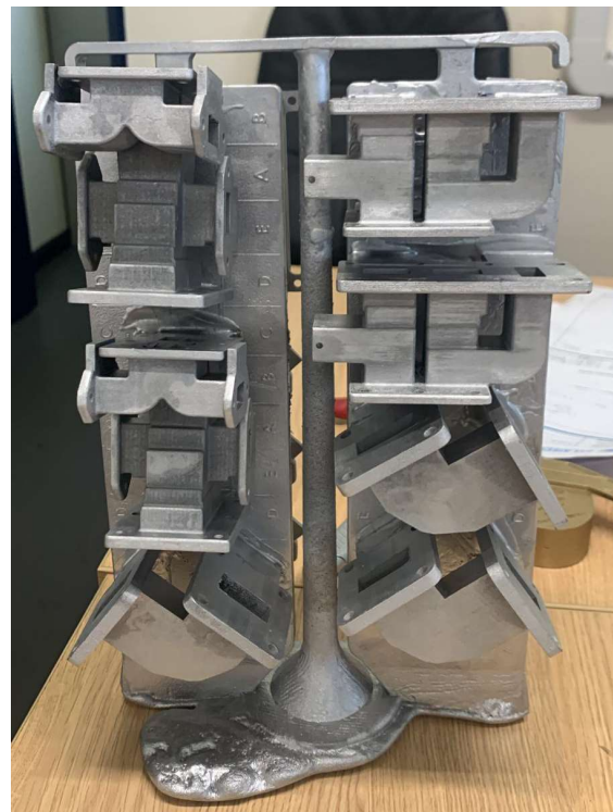
Fig 4 Castings of the 3d printed waxes on the tree
