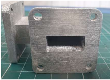
Fig 5 Cast bend manufactured from a 3d printed wax
