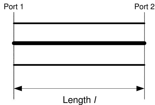
Figure 1: schematic diagram of an air connected between the reference planes of a VNA.
