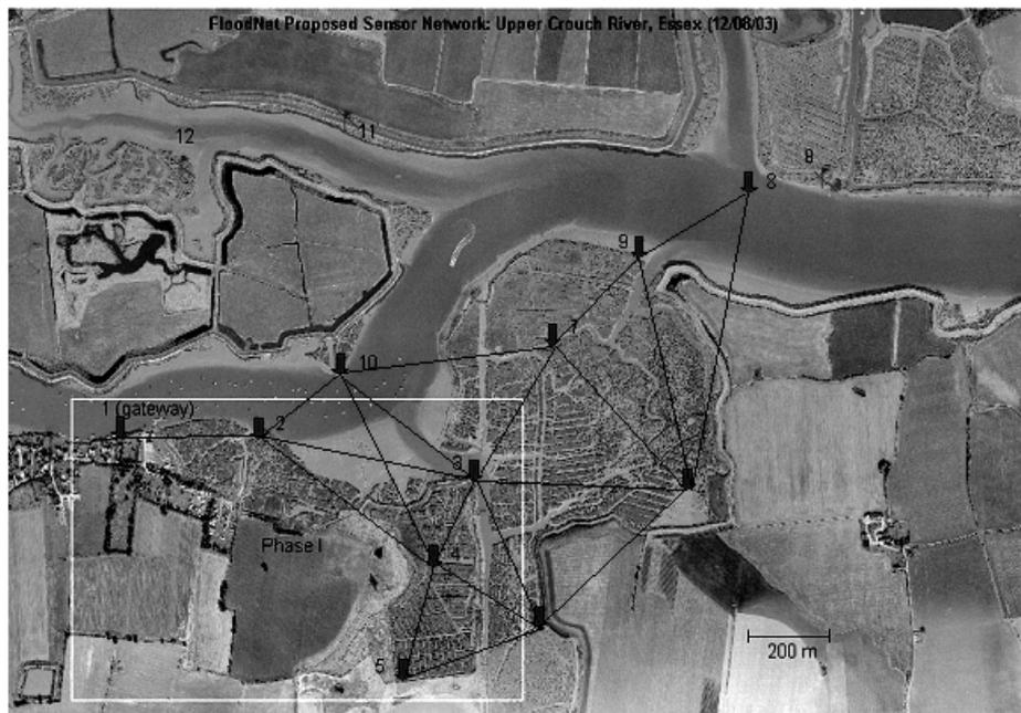
Figure 1: An aerial photograph of the floodplain in Brandy Hole showing the locations of the sensor nodes and the viable communications links between them.
