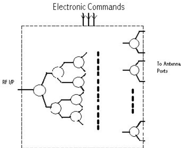
Figure 1 The switched beam forming network.
