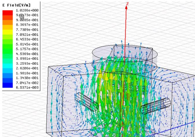
**Figure 3 Electrical field pattern in uncoupled Wye resonators.**
