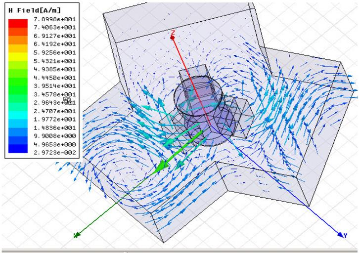
**Figure 5 H-field plot of a waveguide ferrite switch junction.**
