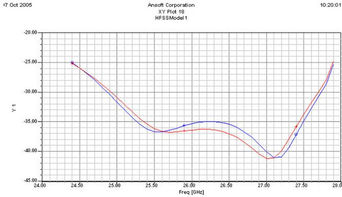
**Figure 6 Isolation/Return Loss plots of the wideband junction.**
