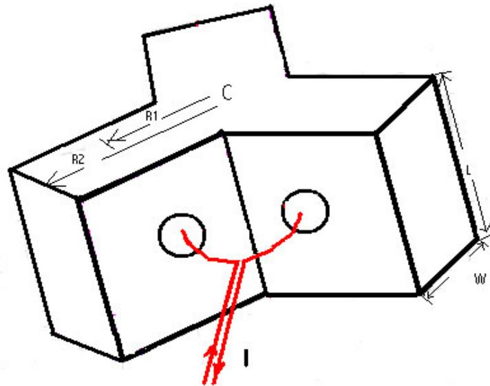
**Figure 2 A WYE Latched Resonator**
