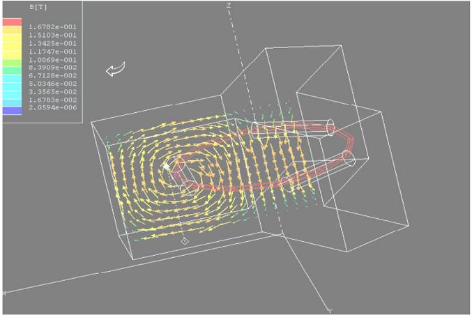
**Figure 4 Static magnetic flux pattern in the latched ferrite.**
