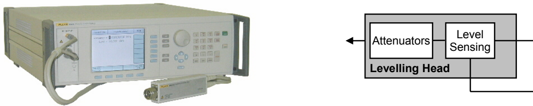
Figure 1. The Fluke 9640A showing the Levelling Head containing levelling and attenuator circuits.
