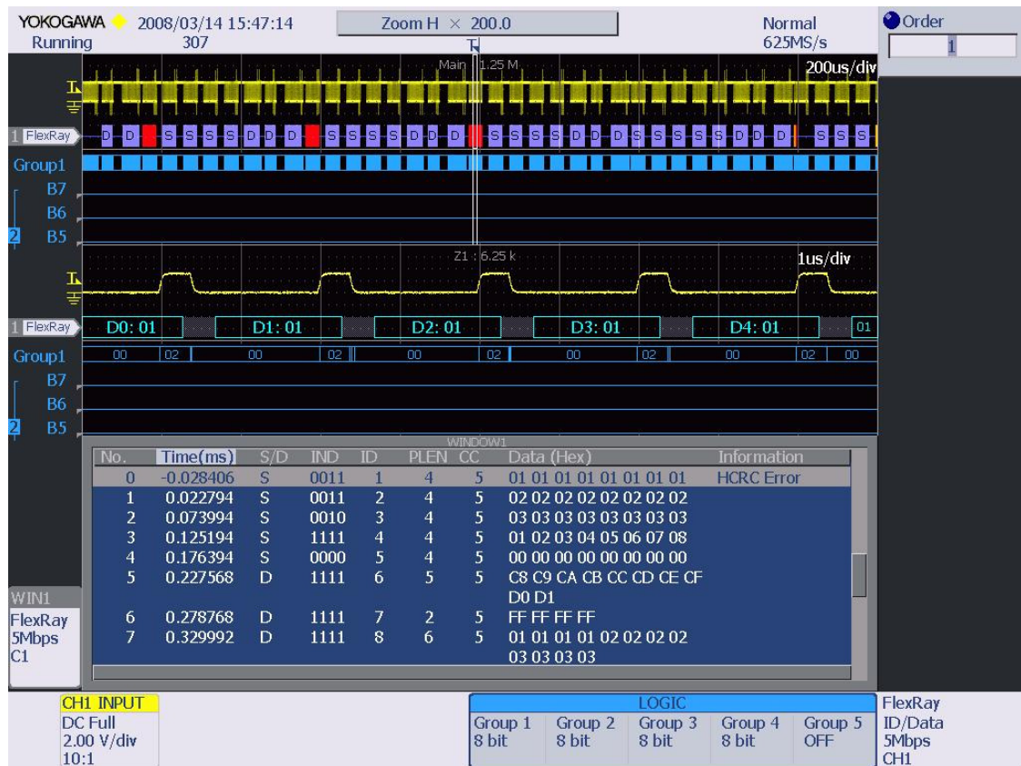
Fig 2. Display showing a single analog channel monitoring a FlexRay bus, while a bundled logic bus is being zoomed in on.
