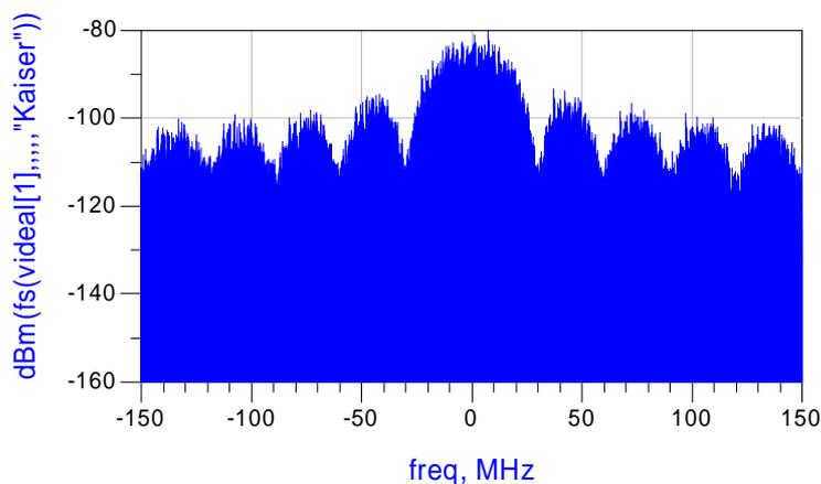
Figure 12 QPSK signal generated by ADS
