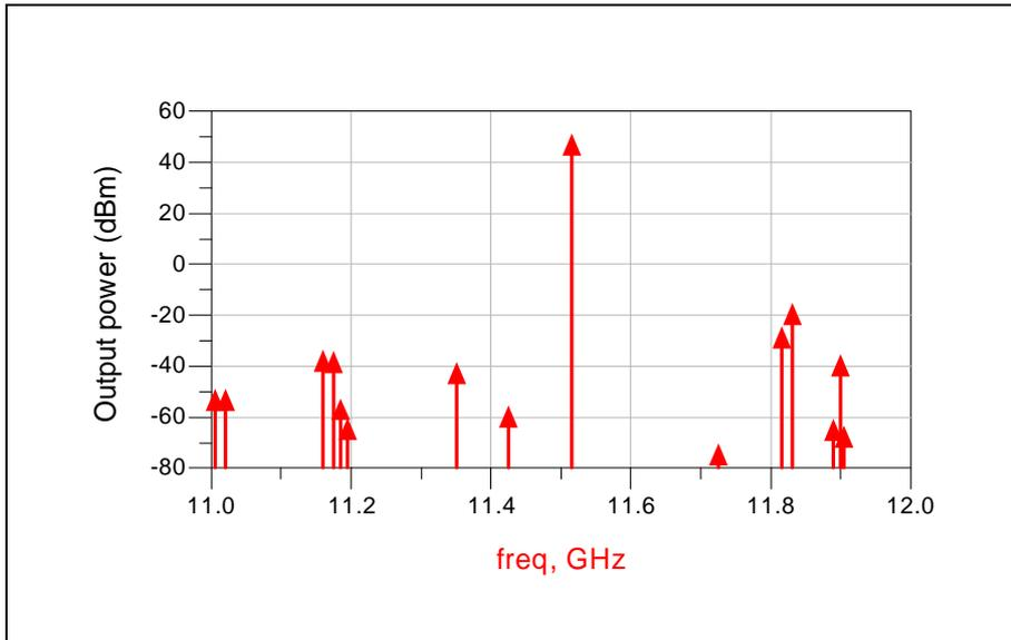
Figure 8 Output carrier related spurious signals from a single input signal
