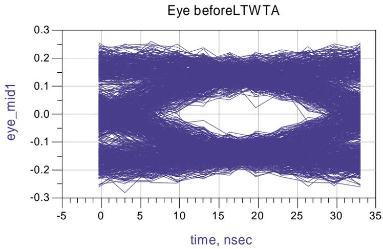
Figure 16 Eye diagram produced by the QPSK signal prior to the LTWTA
