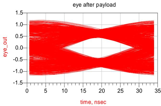
Figure 17 Eye diagram after having passed through the payload and having entered a receiver model
