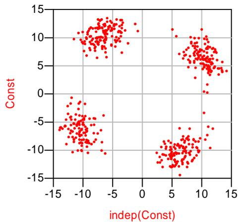
Figure 18 Constellation diagram of the received signal
