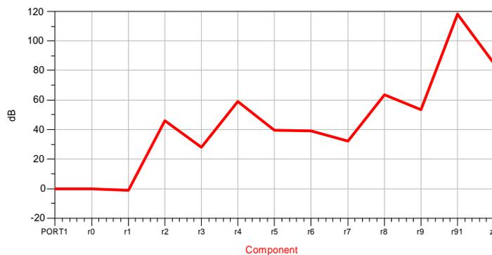
Figure 4 RF signal gain level through the payload
