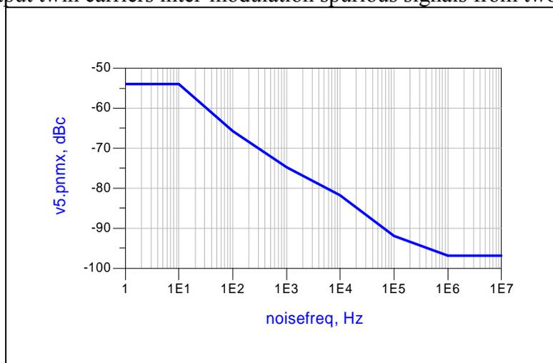
Figure 10 Phase noise of the payload model due phase from each oscillator
