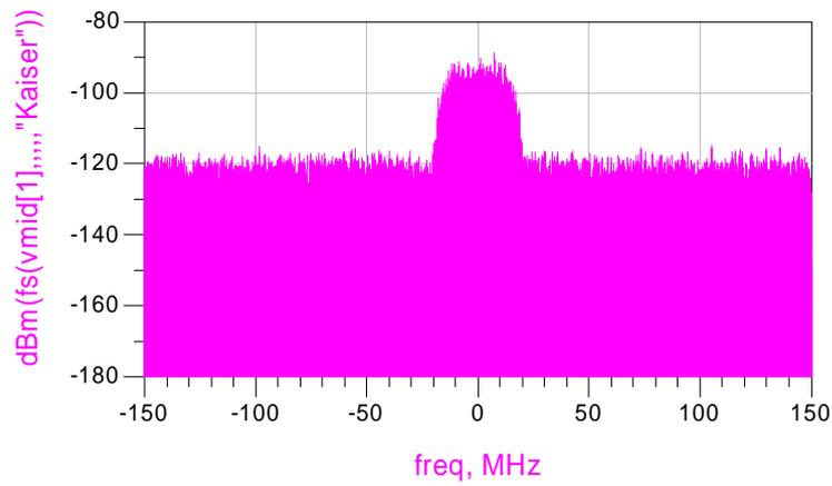
Figure 13 Raised cosine filtered QPSK signal generated by ADS
