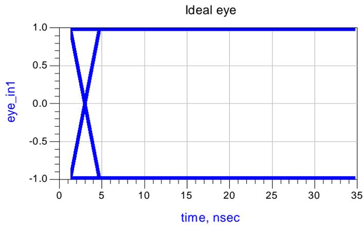
Figure 14 Eye diagram produced from the ideal QPSK signal
