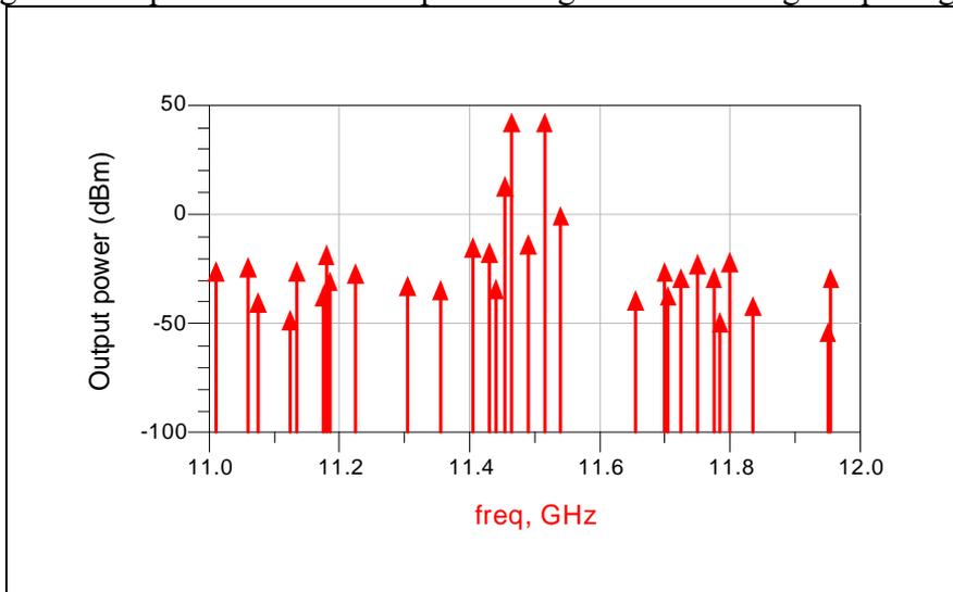
Figure 9 Output twin carriers inter-modulation spurious signals from two input signals
