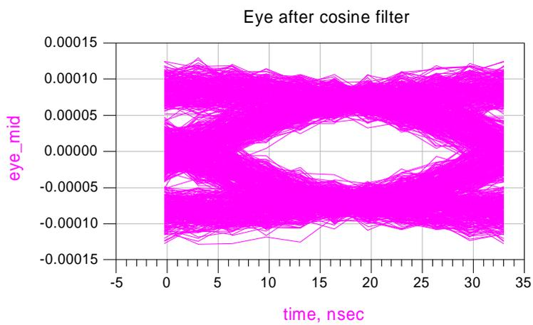
Figure 15 Eye diagram produced by the raised cosine filtered QPSK signal
