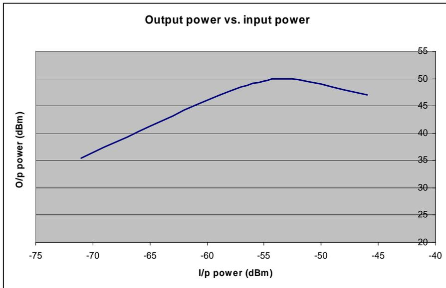
Figure 11 Output power vs. input power of the generic payload
