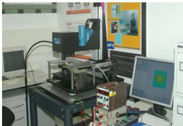
Figure 1: IR thermal microscopy facility at De Montfort University.
