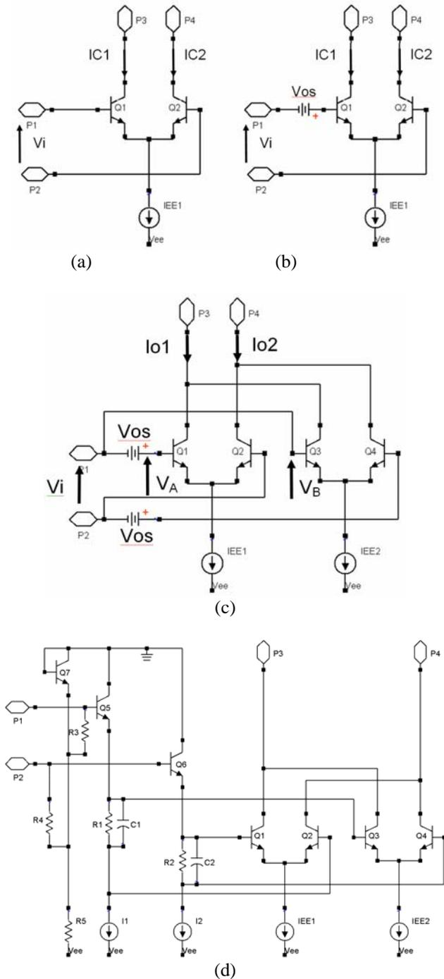
Figure 2 Development stages of a Full wave rectifier circuit from (a) Basic differential pair, (b) Unbalanced differential pair and (c) Two cross coupled unbalanced differential pairs and (d) the circuit implementation used in this design.
