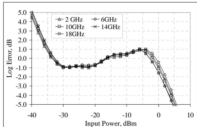
Figure 12: Normalised log error for best fit line at each frequency.
