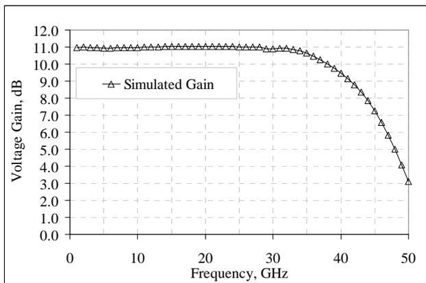
Figure 5 Simulated differential amplifier response
