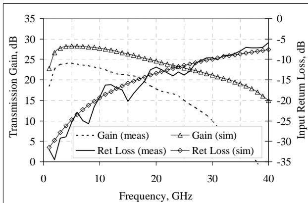
Figure 9 Small signal s-parameters.
