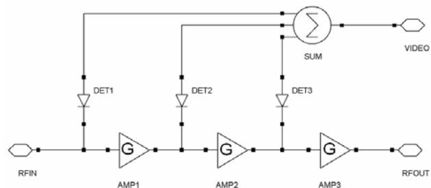
Figure 1 (a) SDLA Block Diagram
