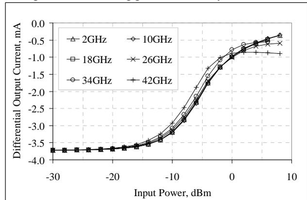
Figure 3 Full wave detector circuit simulated response.
