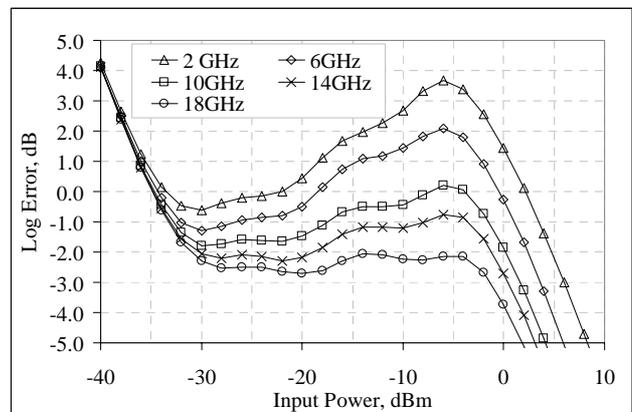
Figure 11: Normalised log error to best fit line of 0.22mA/dB.
