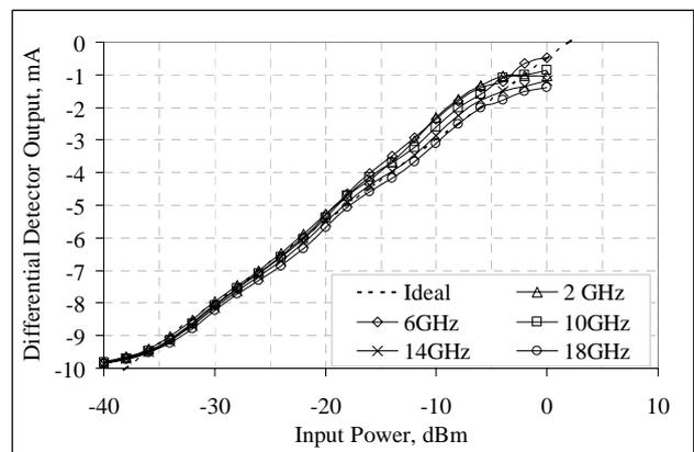
Figure 6 Simulated 3 stage SDLA MMIC transfer characteristic.
