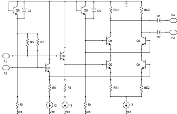
Figure 4 Cascode Differential amplifier configuration.
