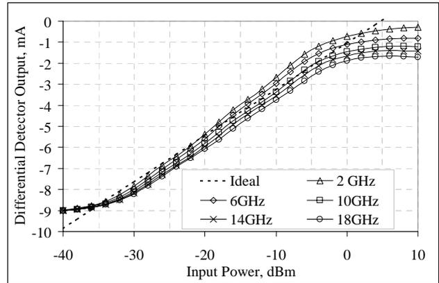
Figure 10: SDLA RFOW Logarithmic transfer characteristic.
