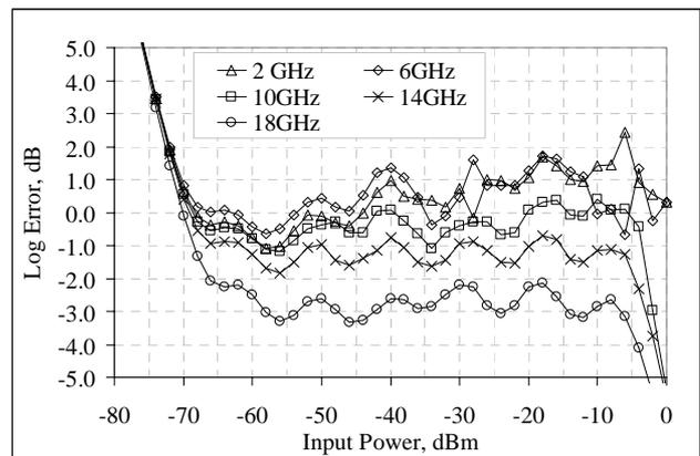
Figure 7 Simulated SDLA Dual MMIC transfer characteristic.
