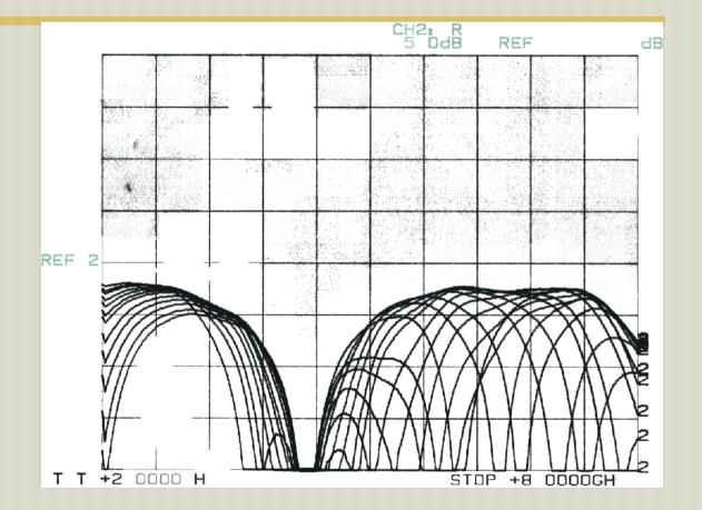
Twin slug tuner shows 2GHz reflection varied up to a limit of 2dB return loss (limited by slug dielectric) with a constant transmission window at 4GHz
