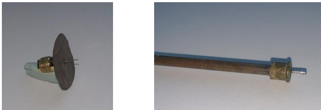
Figure 4 Antennas used in the study (Left) monopole, (right) sleeve dipole
