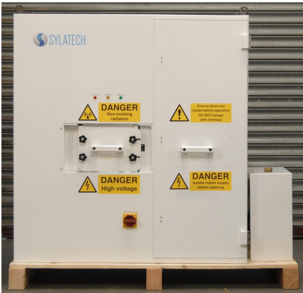
Fig 2 Laboratory scale equipment for microwave pyrolysis
