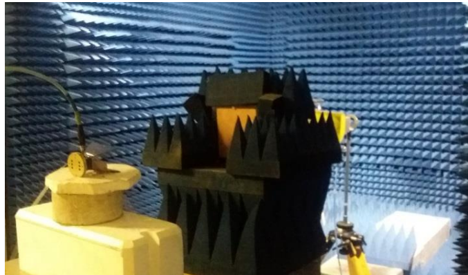
Fig. 13. Experimental setup to measure the transmission coefficient of the FSS.
