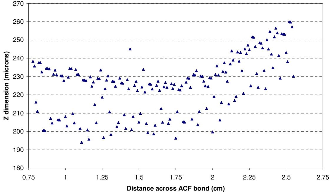
Figure 3: Laser surface scan of grossly misaligned test vehicle showing a variation in height of approximately 30  $\mu\text{m}$
