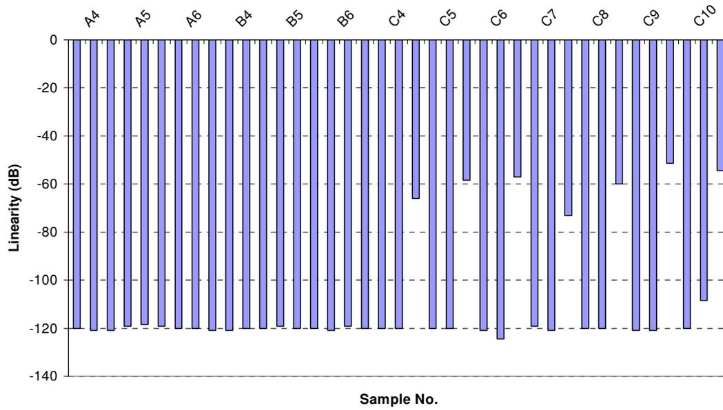
Figure 4: Calculated non-linearity values for three meander sections on a selection of ACF bonded interconnects
