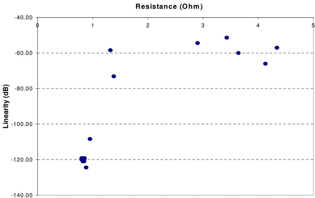
Figure 5: DC resistance of meander sections from C samples plotted against their non-linearity values
