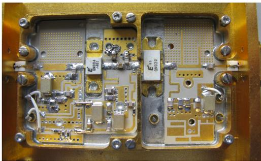
**Fig.3. Two Stage GaN Driver Amplifier Module**
