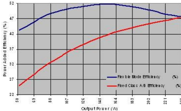
**Fig.7. RF Tray Output Power and Efficiency**
