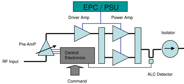
**Fig.2. SSPA Electrical Architecture**
