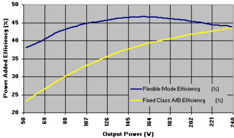
**Fig.8. Output Power and Efficiency of the Complete SSPA in Flexible and Fixed Operating Modes**
