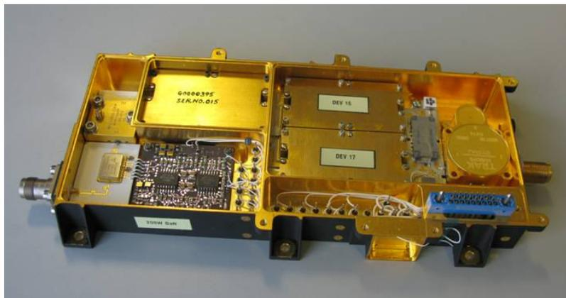
**Fig.5. Photograph of the Complete 240W SSPA RF Tray**
