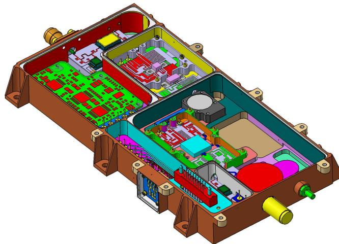
**Fig.9. CAD Layout of Engineering Model 80W S Band RF Tray**
