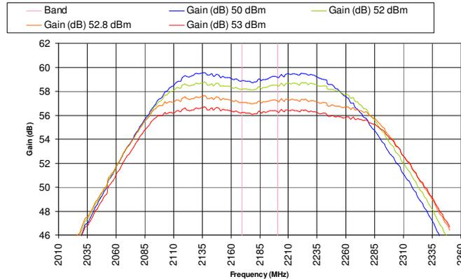
**Fig.6. Measured SSPA RF tray Gain against frequency with 4 different input powers**
