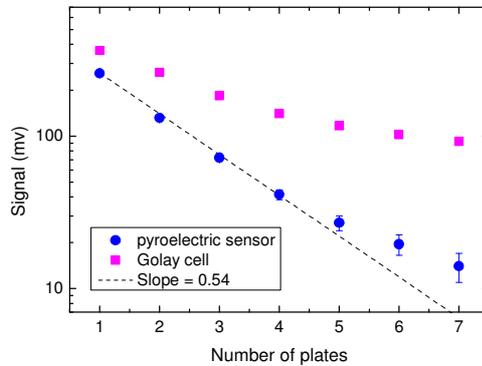
Figure 12. Power linearity tests on a pyroelectric sensor and a Golay cell.
