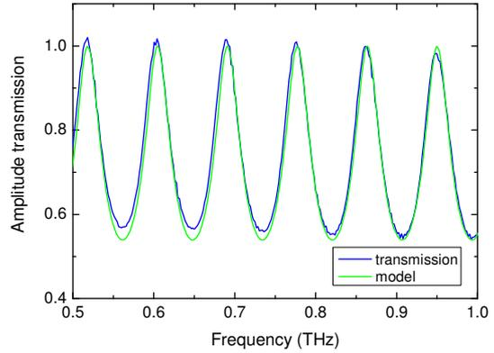
Figure 7. Measured transmission of a Si wafer etalon and model calculated from Eq. 4.
