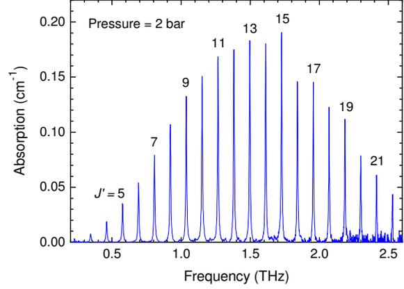
Figure 4. Absorption spectrum of CO (carbon monoxide).
