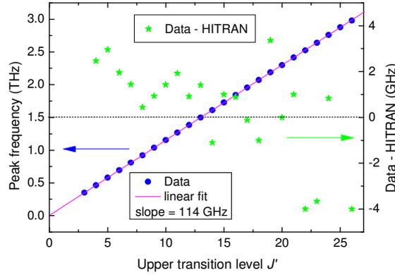
Figure 5. Left: Measured frequencies of CO absorption lines. Right: Deviation from the HITRAN database.
