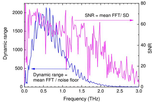
Figure 14. Left: The DR of the amplitude spectrum, calculated as the ratio of the amplitude and the noise floor. Right: The SNR of the amplitude spectrum, calculated as the ratio of the amplitude and its standard deviation.
