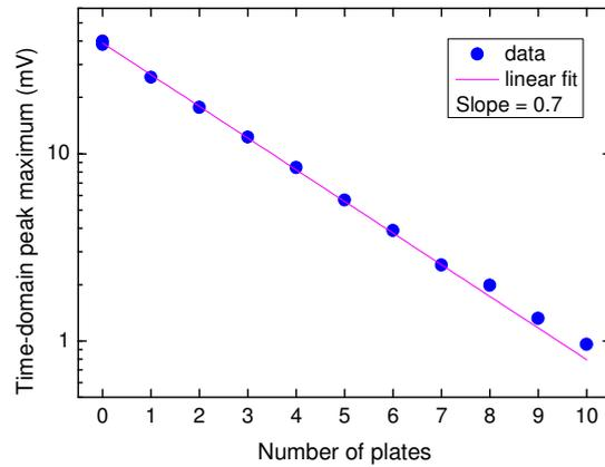
Figure 10. Amplitude linearity test of the time-domain peak maximum (frequency-averaged).
