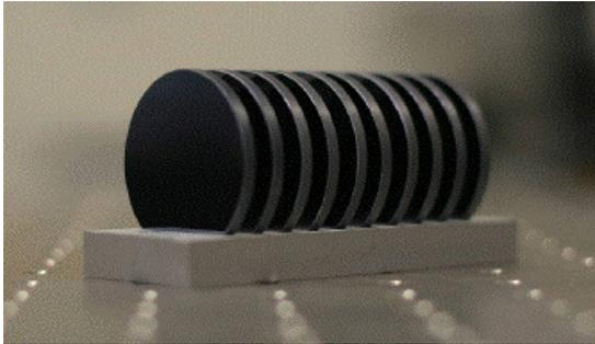
Figure 9. A stack of silicon plates for calibrating the linearity of amplitude measurement.
