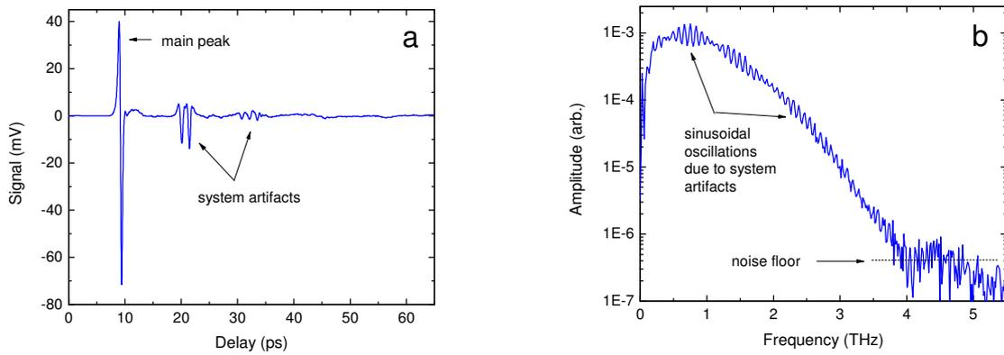
Figure 2. a) A typical time-domain trace. b) Associated THz spectrum calculated by FFT.
