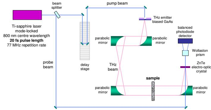
Figure 1. A schematic drawing of the THz TDS employed at NPL.
