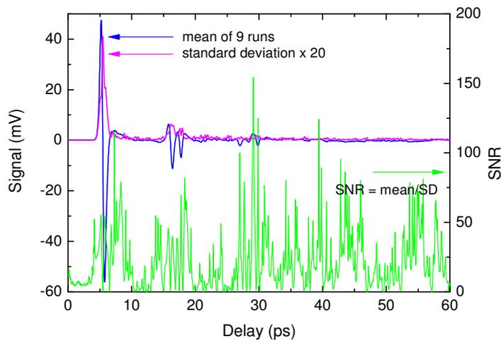
Figure 13. Left: A typical time-domain trace (mean of 9 runs), and the SD of the data. Right: SNR, calculated as the ratio of the mean value and its SD.
