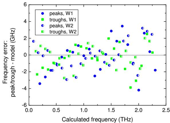
Figure 8. Differences between the measured and calculated peak/trough frequencies for two different Si wafer etalons.
