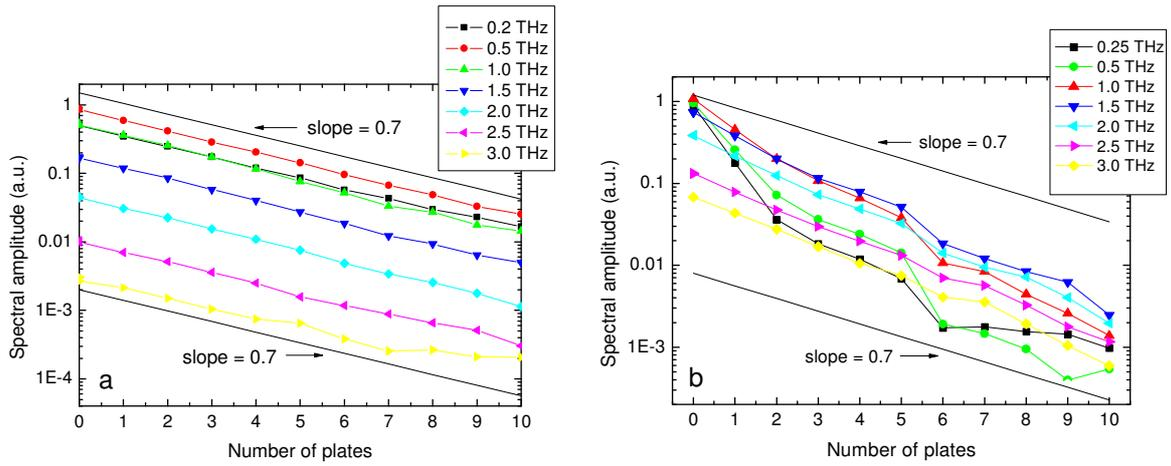
Figure 11. Frequency-resolved linearity tests on a THz TDS: a) after re-alignment, showing satisfactory linearity; b) before re-alignment, showing severe non-linearities.
