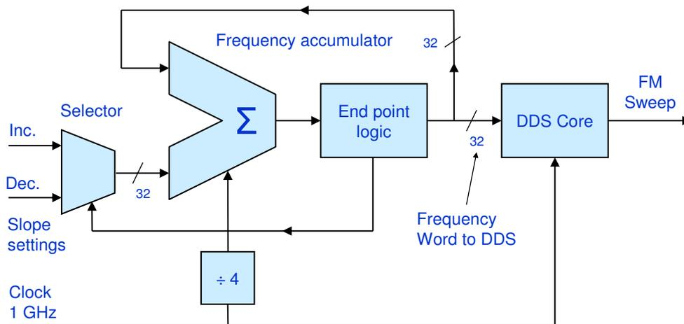
Figure 7 DDS With Frequency Ramp
