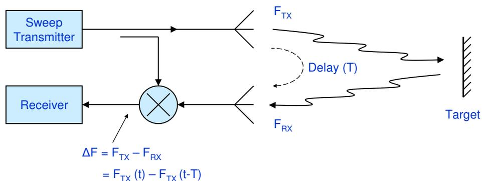
Figure 1 FMCW RADAR Architecture
