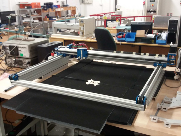
Figure 4: An Inverted E antenna during beam pattern testing in Sylatech X-Y scanner
