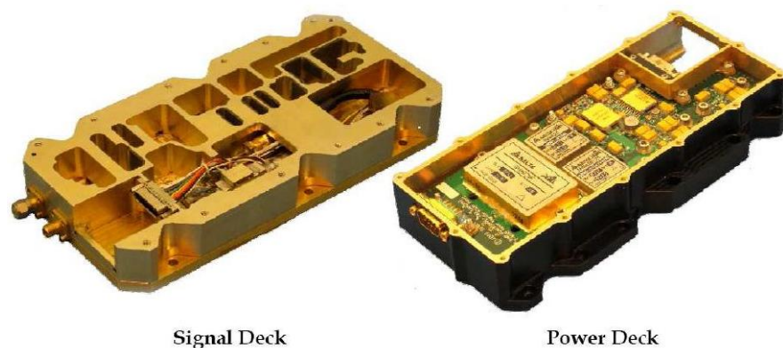
Figure 4: An Illustration of Radiation Hardened Microwave Technology - a Linear X-Band Power Amplifier: image from Space Micro Inc.
