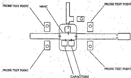
Figure 8 Example of Test Probe Pattern Integrated on Substrate
