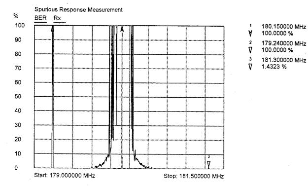
This measurement of an early receiver in the development cycle shows three phenomena. Firstly, spurious signals close to the desired carrier are received to a greater extent than required. This was due to the phase noise profile of the receiver's first local oscillator, which after further investigation was found to be in need of improvement.
