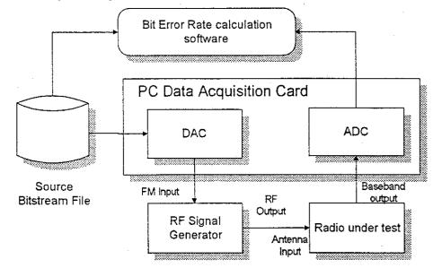
The Bit Error Rate test software is shown below. For small BER measurements, several slots of data can be averaged together to give a cumulative result.
