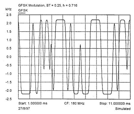
Because of the heavy filtering of the modulating bitstream, the carrier only reaches the maximum deviation of 2.2 kHz when a sequence of ones or zeroes are encountered. Alternating ones and zeroes cause the carrier to remain within 0.5 kHz of the mean carrier frequency. The demodulation algorithm makes use of this property.
