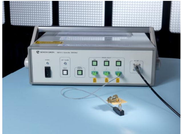
Figure 9. PIFA antenna connected to Electro-optic transducer that is connected to the OEFS controller unit.
