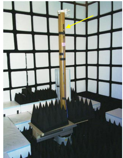
Photo C. Dipole on Kevlar tube, which enclosed plastic roll belt.
