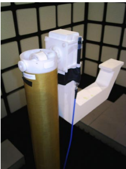
Photo D. Dipole near roll mechanism, worst case. Showing foam platform.
