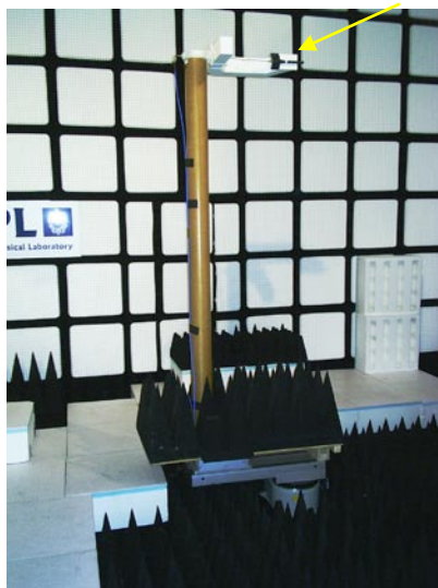
Photo E. Dipole with null facing roll mechanism. Shows bottom surface of foam blocks.
