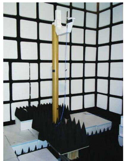
Photo F. Dipole on foam bracket for azimuth scan to give H-plane pattern.
