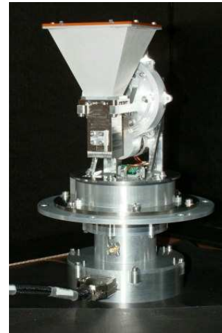
Figure 8 – Antenna pointing mechanism with X-band horn antenna
