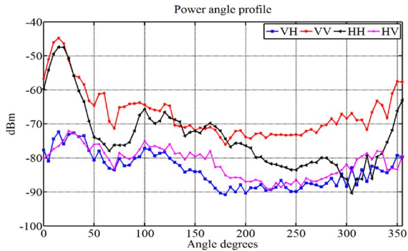
Fig.3 Received power versus angle of rotation for dual polarised measurement in the 67-73 GHz band
