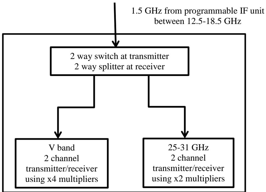
Fig. 1 Block diagram of two transmit by two receive architecture
