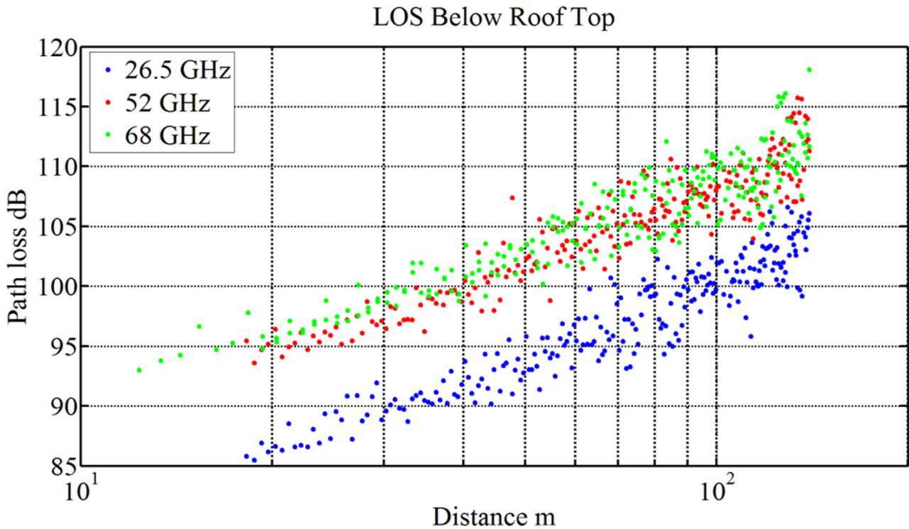
Fig. 4 Path loss versus distance for three frequency bands
