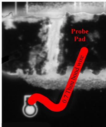
Fig. 7: Thermally isolated micro-cooler
