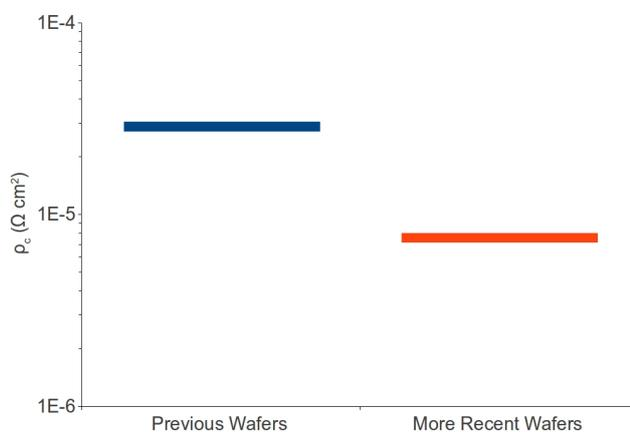
Fig. 9: Improved specific contact resistance on more recent wafers
