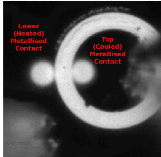
Fig. 6: 10  $\mu\text{m}$  micro-particles on a micro-cooler
