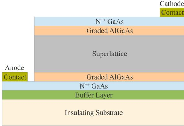
Fig. 3: Basic layer structure of AlGaAs/GaAs superlattice micro-coolers to be characterised
