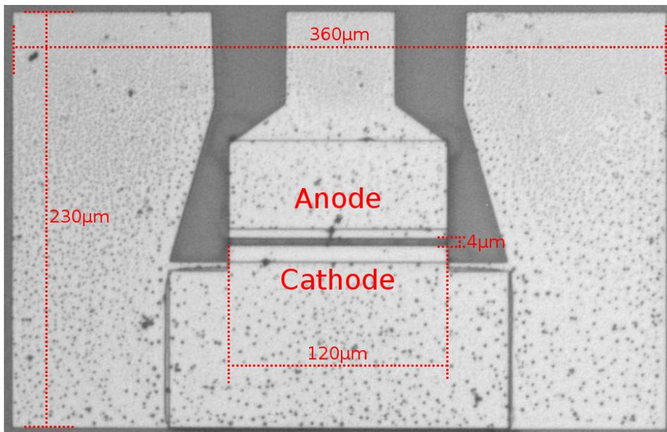
Fig. 2: Planar Gunn Diode with a  $4 \times 120 \mu\text{m}$  channel, fabricated at University of Glasgow
