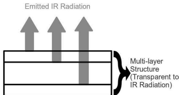
Fig. 4: Multi-layer IR emissions for transparent materials
