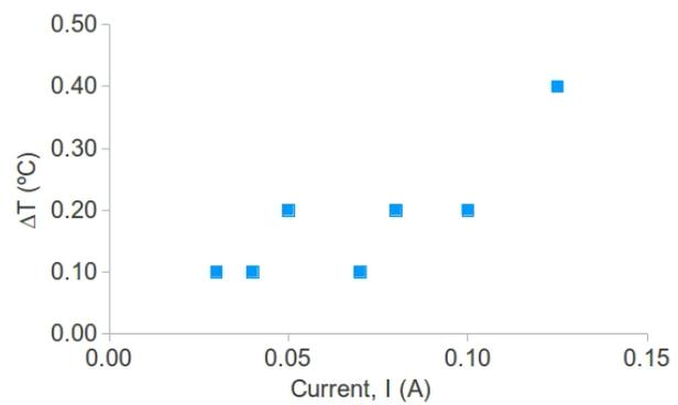
Fig. 8: Cooling ( $\Delta T$ ) against bias current for cooling in Figure 6
