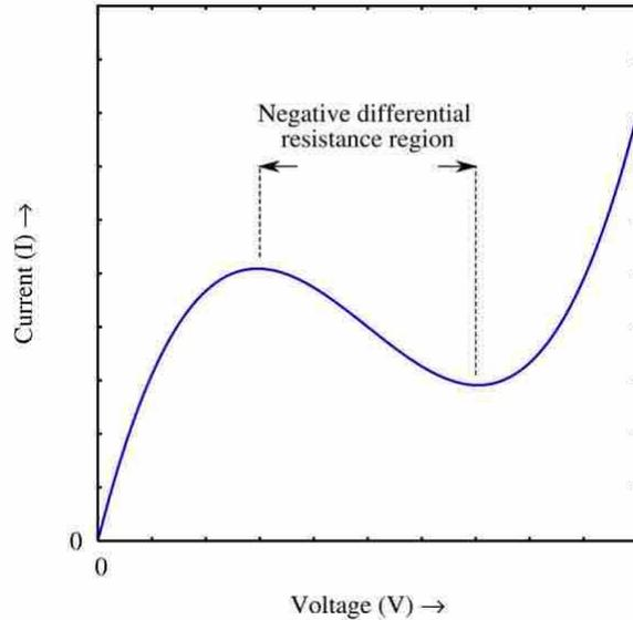
Fig. 1: Approximate Gunn VI characteristic, showing the negative differential resistance region
