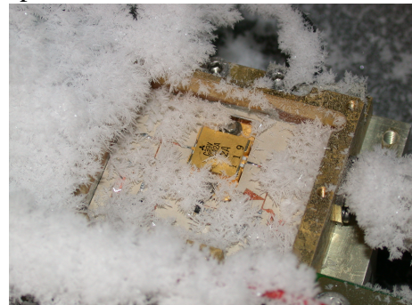
Figure 6 Cold FET in operation
