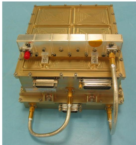
**Figure 6 Complete X-Band Transmitter**
