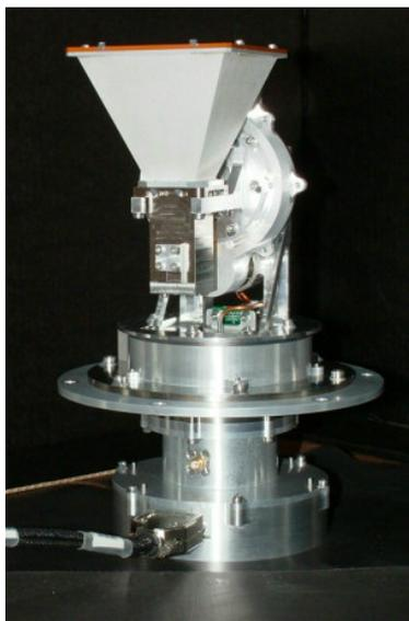
**Figure 8 The Antenna Pointing Mechanism**
