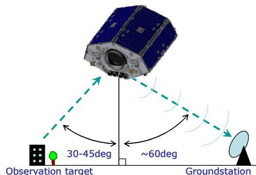
**Figure 7 Agile Downlink Requirement**
