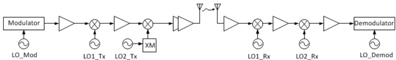
**Figure 2.** Typical satellite link.
