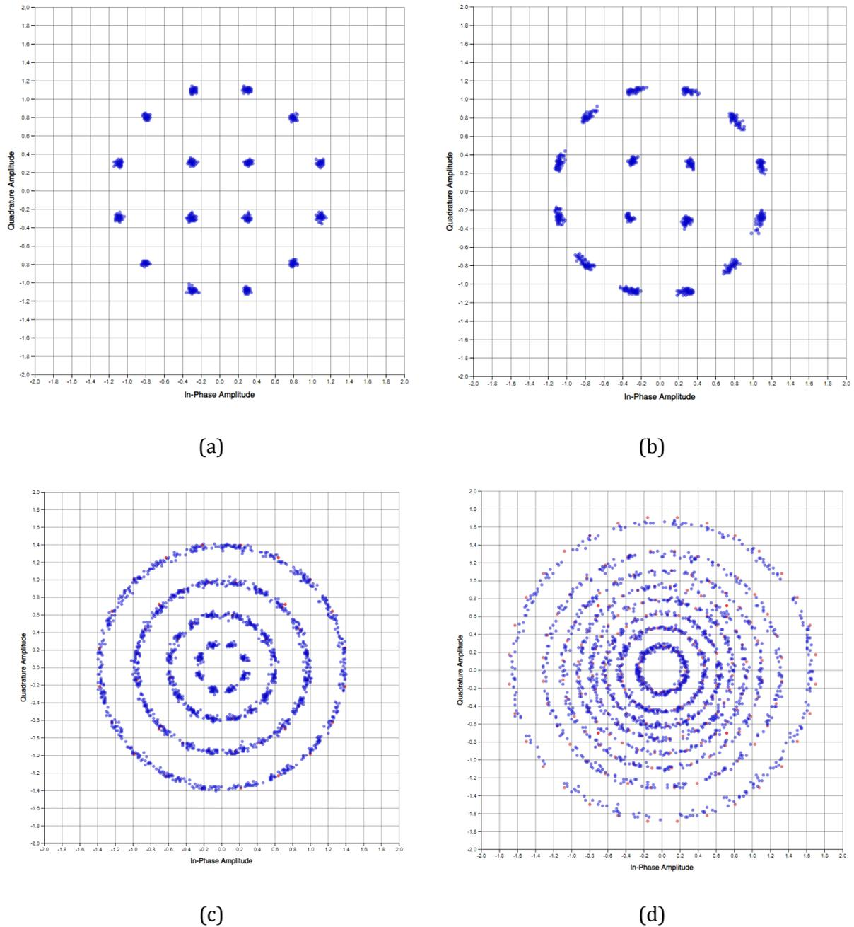
**Figure 4.** Measurement results with a modem a) 16 APSK with modem-to-modem test, b) 16 APSK with Ka-band satellite link, c) 64 APSK with satellite link, d) 256 APSK with satellite link.
