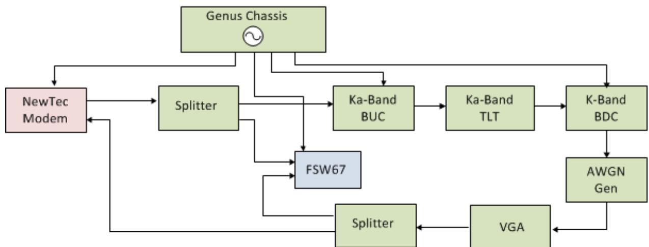
**Figure 3.** Measurement system.
