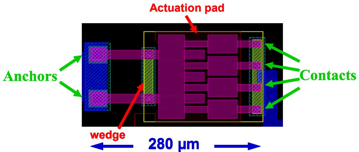
Figure 1: Schematic view of the RF-MEMS switch device.
