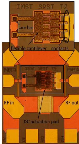
Figure 3: Coplanar SPST RF-MEMS switch processed at OMMIC.
