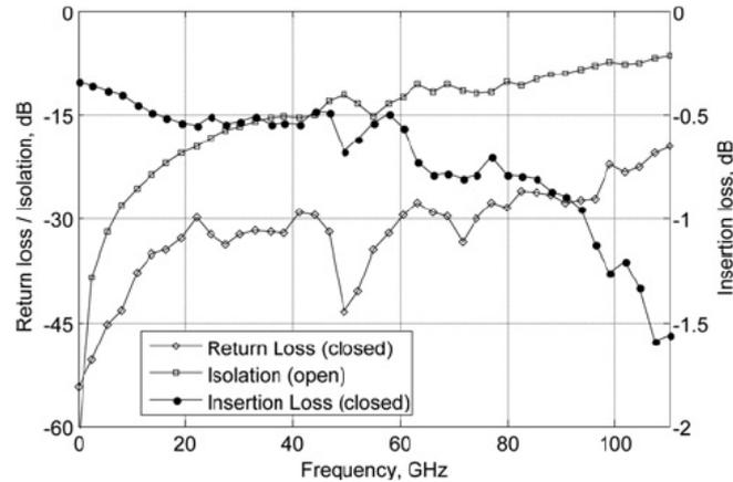
Figure 6: S-parameters measurements of the RF-MEMS SPST up to 110GHz [4].
