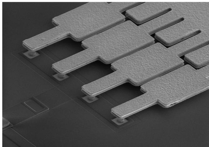
Figure 2: SEM view of the switch processed at OMMIC.
