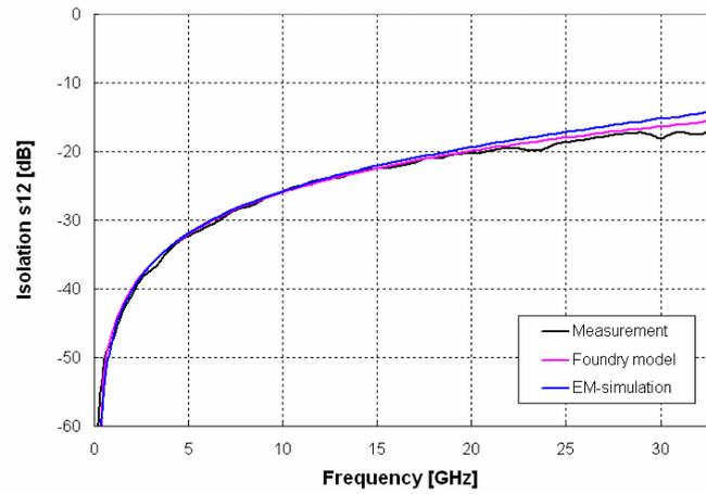
Figure 4: Isolation of the RF-MEMS switch of fig. 3 in the open state.
