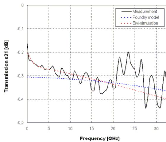
Figure 5: Insertion losses of the RF-MEMS switch of fig. 3 in the closed state.
