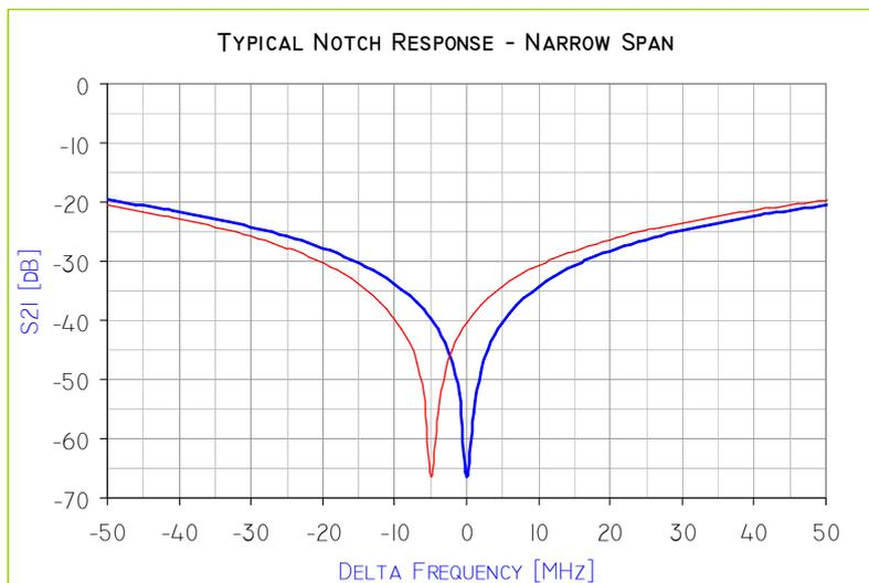
Figure 4. A notch setting compared with 5 MHz drift
