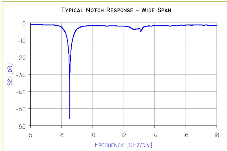
Figure 1. X-band notch filter tuned to 8.5GHz
