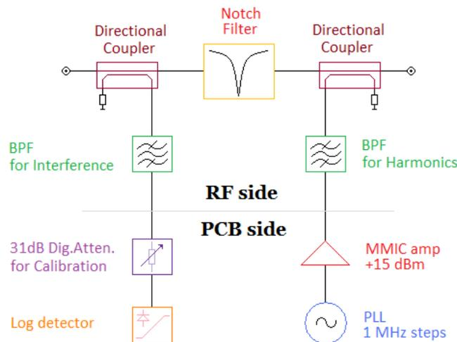
Figure 6. Auto-correction circuit (BITE)
