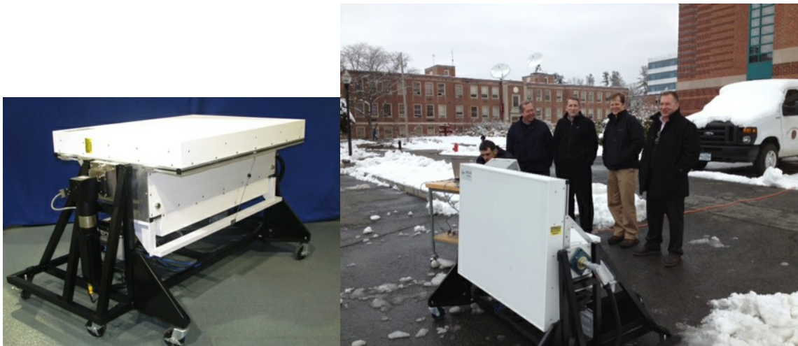
Figure 11. Commercial FRF-166 Phase Tilt Array from First RF Corp. The array electronically scans plus/minus 45 degrees from broadside in the azimuth direction and mechanically tilts over 90 degrees in elevation enabling beam pointing toward the horizon (right) up to zenith (left).
