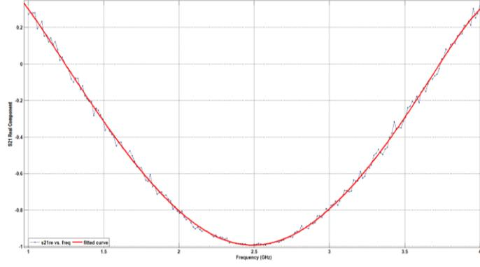
**Figure 2** Curve fitting of real component of transmission scattering parameter ( $S_{21}$ ); blue line represents the original measurement and red line represents the fitted curve
