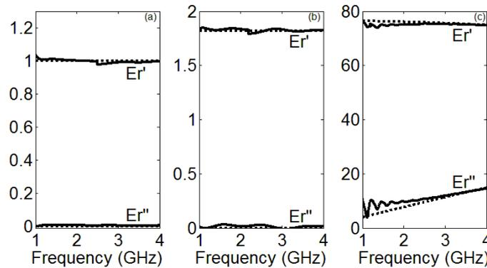
**Figure 3** Complex relative permittivity of (a) Air (b) Teflon and (c) Water; solid line represents measurements and dotted line represents figures from National Institute of Standards and Technology [10]
