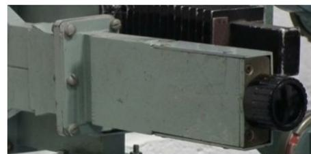
Figure 10 Dual Short-Circuit Phase Adjuster
